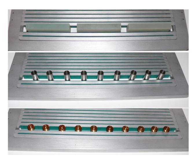
The AHP is capable of handling and positioning parts with different and unusual shapes and sizes, many that cannot be easily handled using standard carrier plates. Parts that are round, square, rectangular, hexagonal, octagonal, thin, thick and odd shapes can be captured with the AHP . This capability allows the use of this technology for numerous applications in addition to MLCC termination. The photos above illustrate some of the possibilities.
