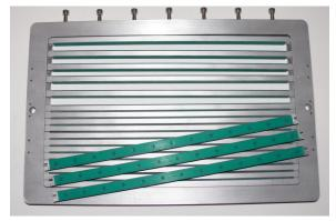
The AHP is a versatile tool. The ability for the user to adjust the number of ribs in the plate reduces the need to purchase different plates for each new chip thickness or size, so the requirement to purchase and maintain many different carrier plates is greatly reduced.
